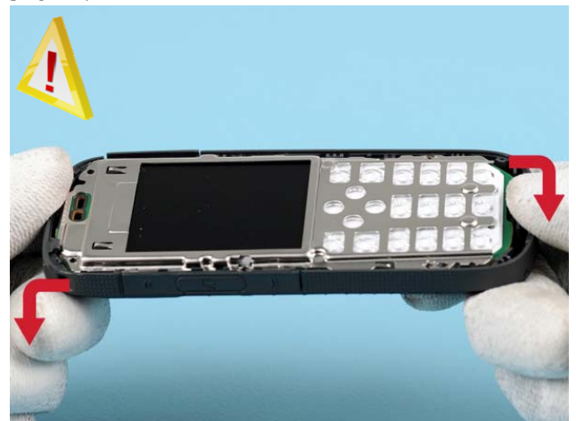
8) There are 4 clips on each side and 2 clips on top of the D-cover. Release the clips by carefully stretching the D-cover out.
