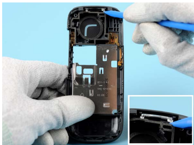
23) Use the SS-93 tool to release the clips holding the TORCH WINDOW.
