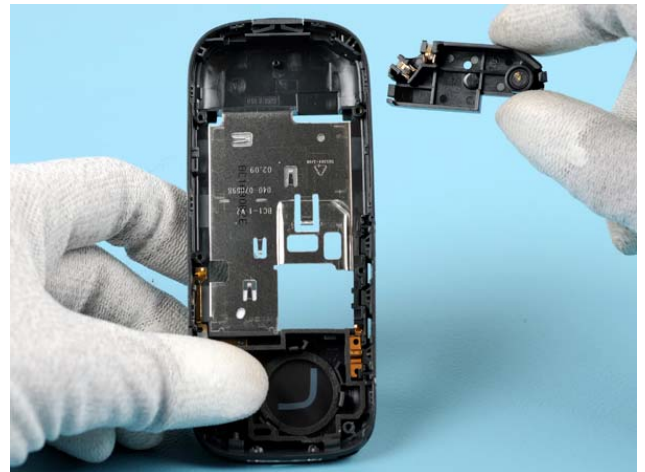
20) Remove the ANTENNA ASSY.
