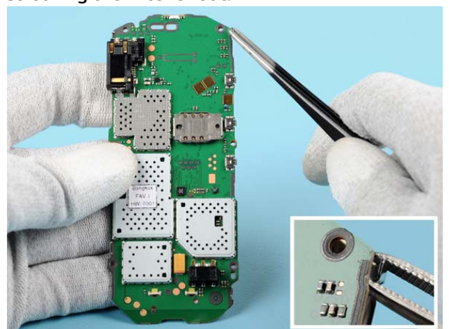
10) Use the tweezers to release the clips on the bottom side and top side (2 on each side) of the engine module.
