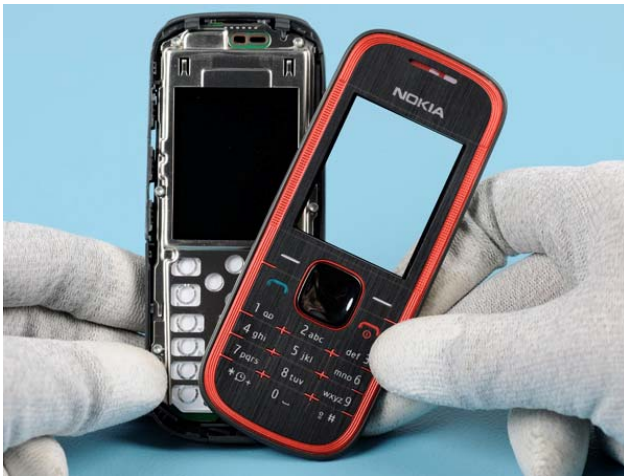
5) Lift up the A-COVER to remove it.
