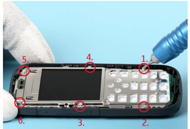
6) Unscrew the 6ea. #4 TORX screws in the order shown.
